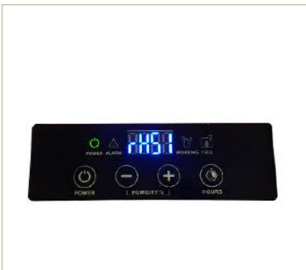
Digital display with reading of ambient and set humidity
