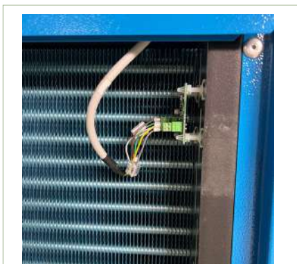
Temperature/humidity electronic board
